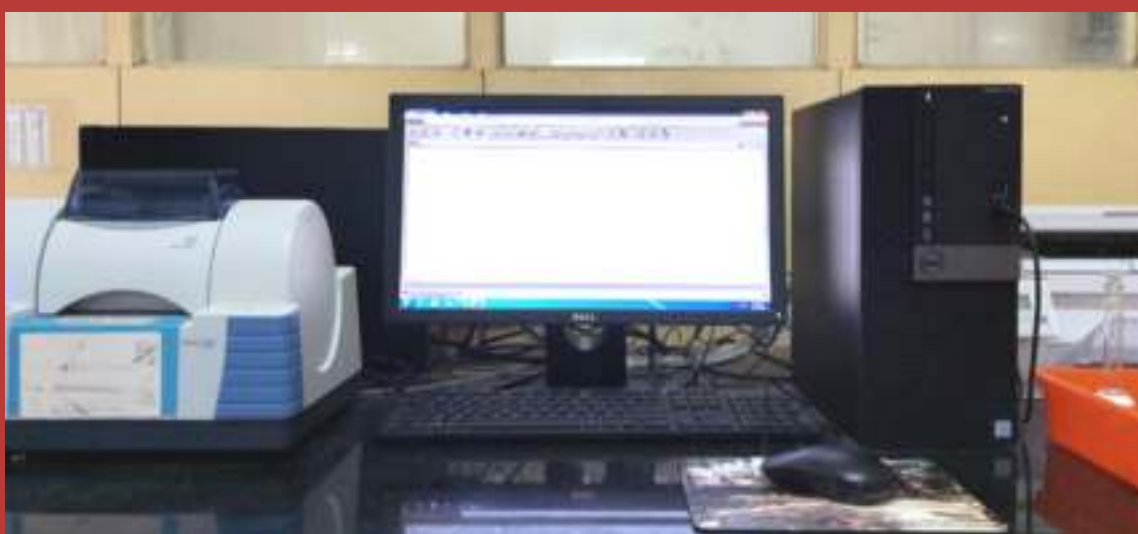
FTIR for mineral oil test, Instrumentation Section, Chemical Laboratory ,SROL
