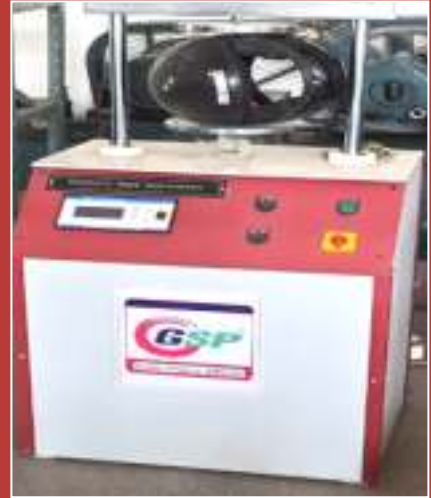
Rigidity Test Setup for testing of Helmets
