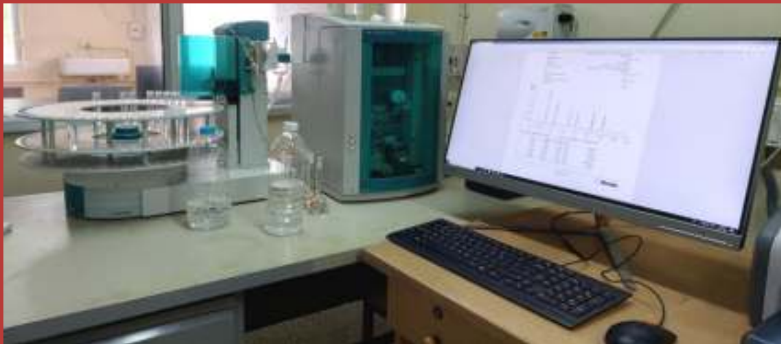
Ion Exchange Chromatograph for bromate test, Instrumentation Section, Chemical Laboratory ,SROL
