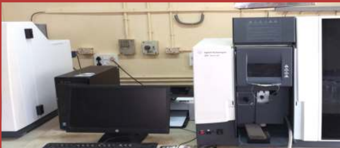
Atomic Absorption Spectrophotometer for testing Packaged Drinking Water, Instrumentation Section, Chemical Laboratory ,SROL
