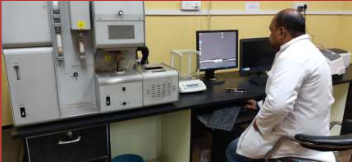
Carbon Sulphur evaluation in steel, Chemical Section, NROL
