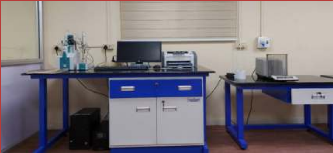
Potentiometric Auto Titration for testing Silver, Instrumentation Section, Chemical Laboratory ,SROL
