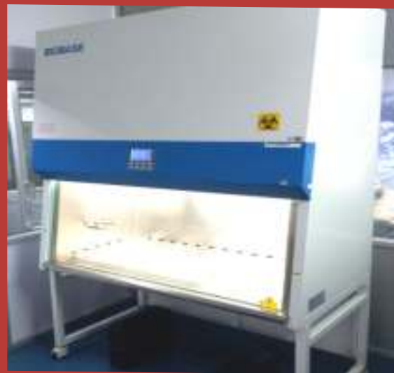
Biosafety Cabinet Level 2 For handling Pathogen, Microbiology Lab, SROL
