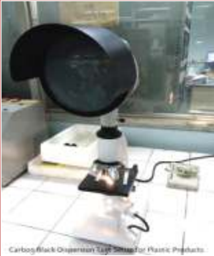
Carbon Black Dispersion Test Setup for testing of Plastic Products
