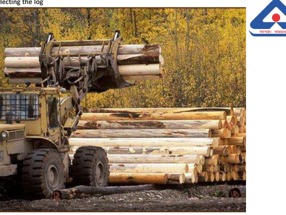
The initial step in manufacturing plywood is selecting the logs. Logs are chosen according to its physical properties. Maturity, straightness, and roundness are the most critical factors to be considered in selecting raw logs. Plywood manufacturers also ensure that all raw logs used in plywood come from a legal source and sustainable forest concession.
