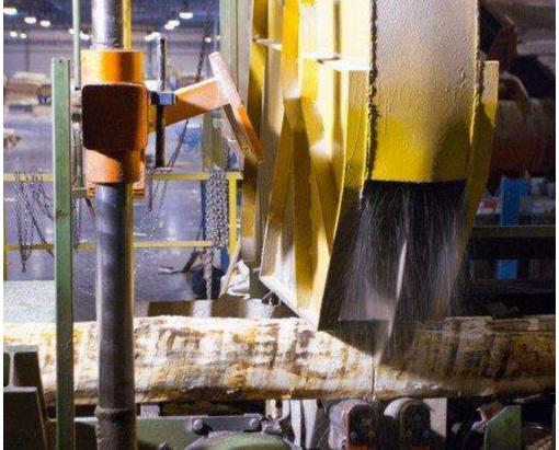
After the debarking process, the logs are cut into desired lengths in step known as bucking. This process is done so that the next operation which is peeling the bark can be efficiently executed.
