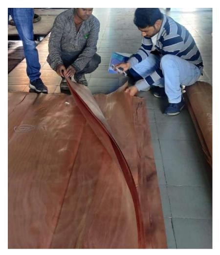
The face veneer was then coded with unique code and signed and also counter sign was obtained from firm, to ensure traceability of that veneer.
