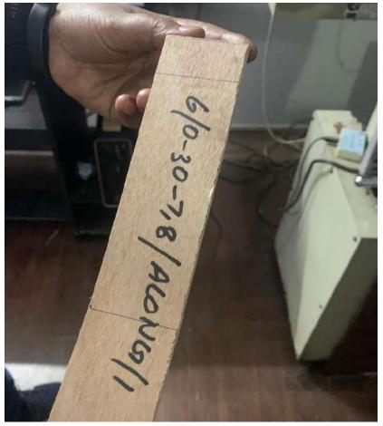
4. The specimen was then preconditioned to a constant mass at a relative humidity of 65 ± 5 percent and at a temperature of 27 ± 2°C and then taken up for testing of Modulus of Rupture (MOR) and Modulus of Elasticity (MOE) by Central Loading Method.
