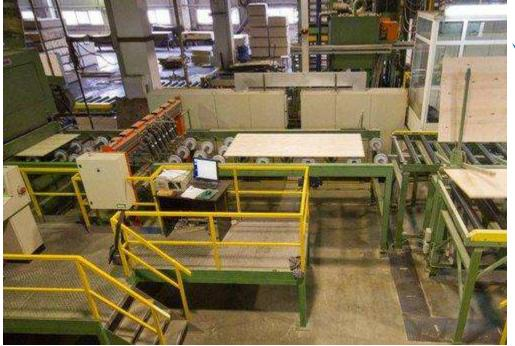
The sheet will undergo processes to make it presentable and saleable in the market. These methods include trimming, sanding, and finishing. Because of these processes, the sheets takes down into standard sizes which meet the needs of the customers. Also, these processes are the reason why plywood seen in the market has smooth edges and texture. The finished plywood products are divided into two categories indicating whether it is for exterior or interior used.
