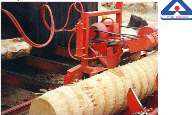
The second step is the debarking process. Logs are feed into a debarking machine. Just like shown in the picture. As the logs rotate from the ridged wheels, the cutting head on the track is reversely rotating with the log from end to end, causing the bark to be removed. The purpose of this is to peel the bark without damaging the wood.
