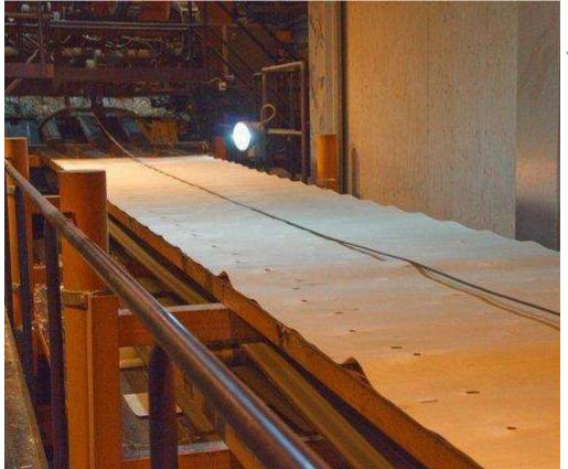
After peeling, the next method to be done is creating a continuous ribbon of wood. The log rotates and feeds towards the cutting edge of the lathe creating continuous and unwounded thin layers of wood. The thickness of the veneer depends upon how it is used.
