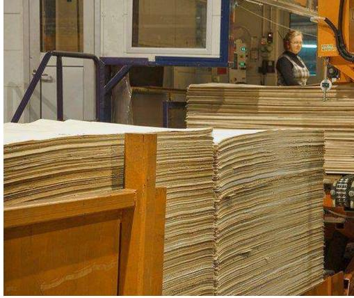
The piece of wood is cut to a standard size of 4' x 8'. The ideal thickness of plywood range from 1/4'' to  $3\frac{1}{4}$ , but the actual thickness of the plywood after production is determined after the sheets are pressed and glued together. The sheets are automatically scanned as it comes up in the peeler. After scanning, it is stack in preparation for transferring and drying using drying ovens.
