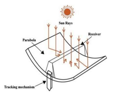
This is one of the versatile systems that can be used for desalination, steam and power generation. The fluids inside the system reaches about 200°C.
