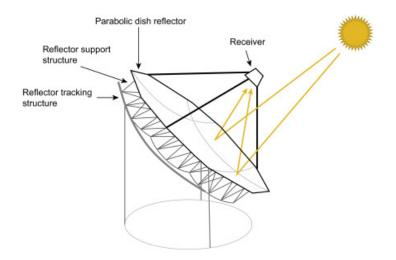
This system can generate high temperatures of about 350°C and finds application in power generation through operating a Stirling engine and steam generation.
