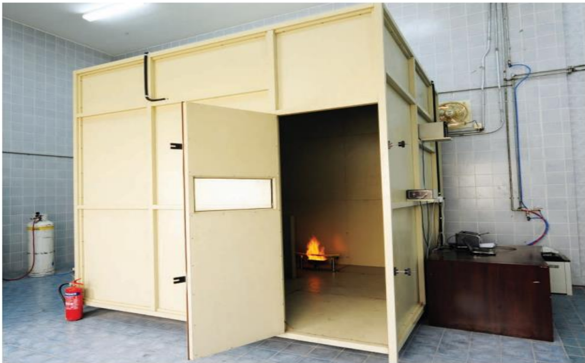
Smoke density 3 m test cube (IEC 61034)
