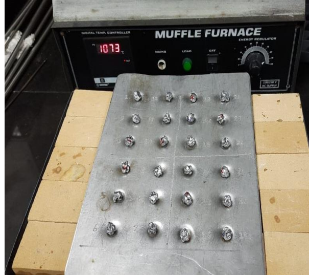
Figure 4: Assay and the Proof Assay samples for feeding in to Cupellation furnace
