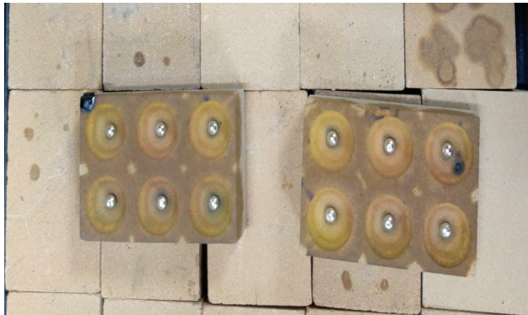
Figure 6: Completion of Cupellation process
