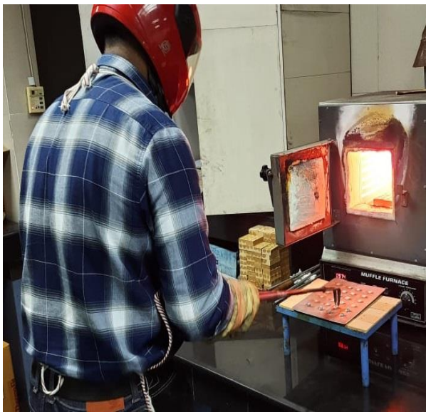
Figure 5: Assay and the Proof Assay samples feeding in Cupellation furnace
