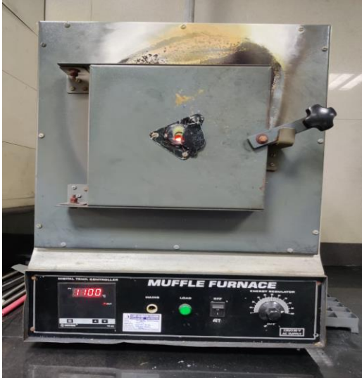
Figure 3: Pre-heating of Cuples in Cupellation Furnace
