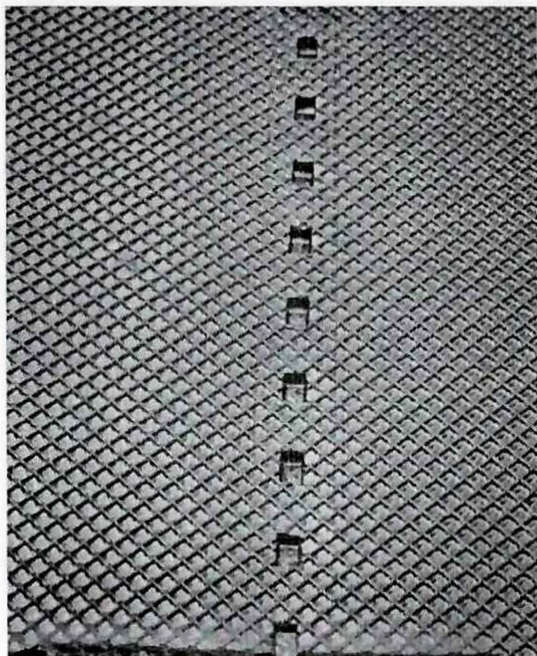
FIG. 5 (a) ULTRASONIC SEAM WELD
