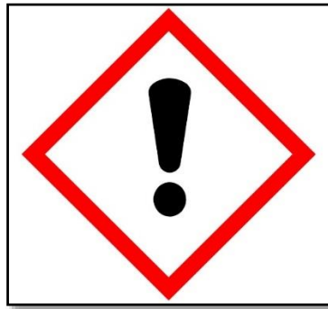
FIG. 1 INDICATES CAN CAUSE CERTAIN HEALTH EFFECTS FOR EXAMPLE, SKIN IRRITATION, EYE IRRITATION, ETC
