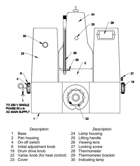
Fig. 2 Torsion Balance Moisture Meter (0 - 100 percent) Front View
