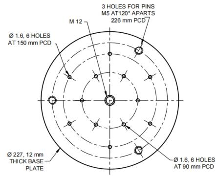
3A SURCHARGE BASE PLATE (FOR MOULD 3 000 cm<sup>3</sup>)
