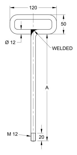
A = 275 mm for mould of capacity 3 000 cm<sup>3</sup> A = 200 mm for mould of capacity 15 000 cm<sup>3</sup>
