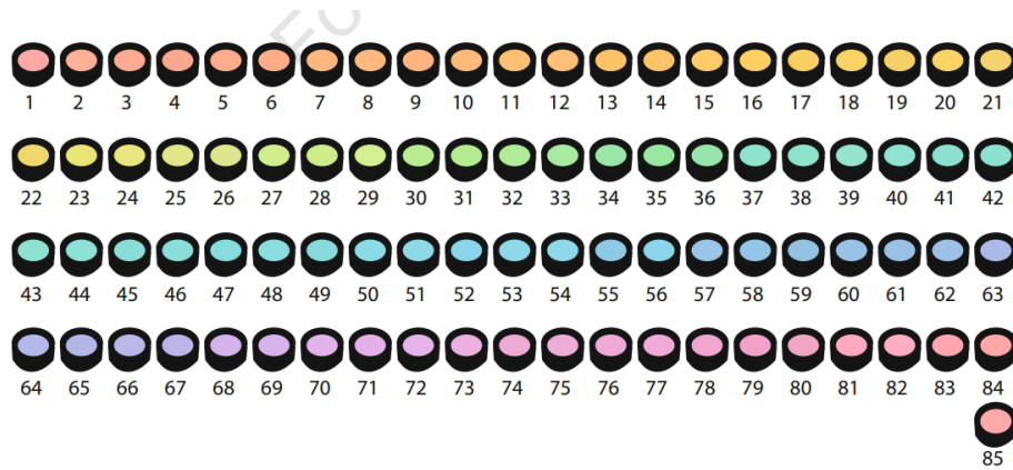
Fig. 17 Farnsworth-Munsell 100 hue (FM100) test cylinders *
