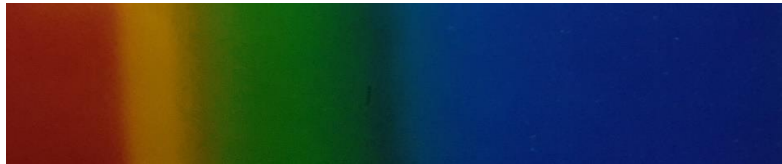
Fig. 15 Spectrum of Black Body Radiator the Continuous Spectrum for Thermal Radiator (Halogen Lamp 3000k)
