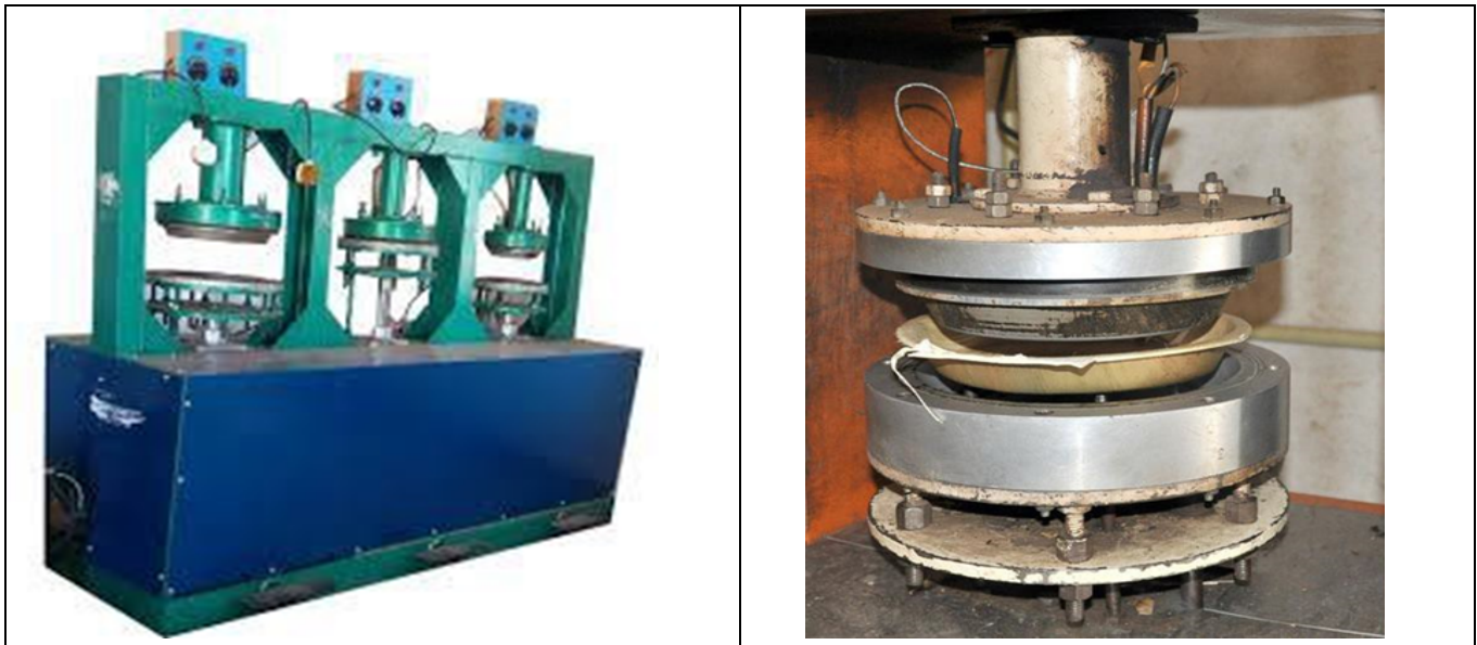
FIG.3 HOT PRESS FOR MAKING LEAF PLATES
