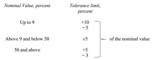
The actual value of copper content shall he calculated to two decimal places and then rounded off to one decimal place before applying the tolerance.
