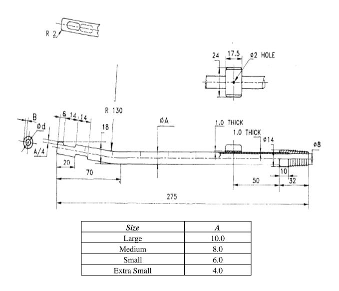
NOTE - Dimensions 'B' shall depend on dia 'A' to get maximum diameter 'd'. However, the tip shall be rounded off smoother and free of any sharp edges.
