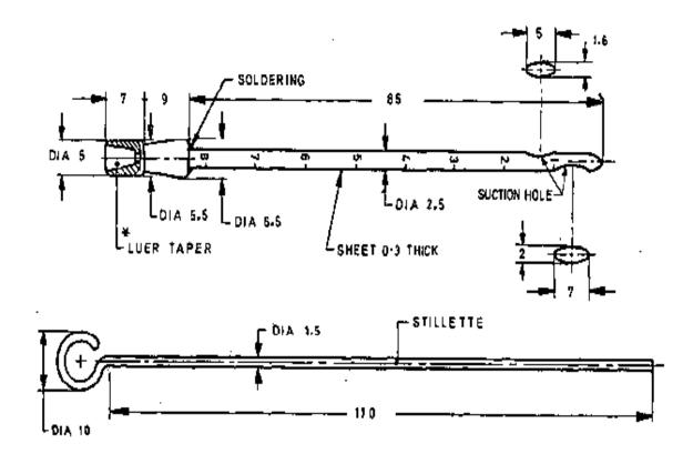
All dimensions in millimetres. FIG. 1 BRAIN CANNULA
