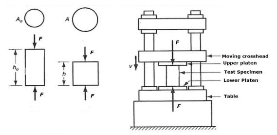
A<sub>0</sub> initial area of test specimen
