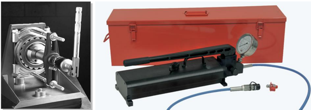
FIG. 35 PULLER WITH HYDRAULIC ASSIST
