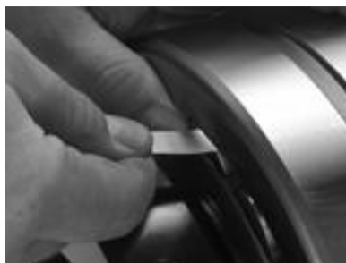
FIG. 15 CHECKING DIAMETRIC SLACKNESS BY FEELER GAUGE
