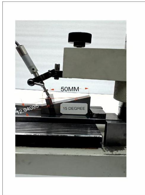
FIG. 5 CALIBRATION OF ANGLE GAUGE USING COMPARATOR STAND
