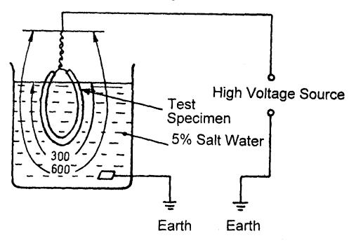
All Dimension In Millimetres. Fig.1 Immersion Test Plan
