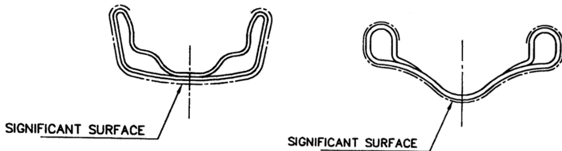
FIG. 13 SECTION OF RIM SHOWING SIGNIFICANT SURFACE OF ELECTROPLATING
