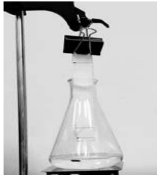
FIG 9 SPECIMEN PREPARED FOR VERTICAL WICKING TESTING IN AN ERLLENMEYER FLASK
