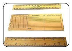
**Sizes & Types:** Four types (A, B, C, D) with specific sizes. B and C have three scales (1:100,000; 1:50,000; 1:25,000), D has (1:100,000; 1:8,000; 1:4,000), and A has one scale (1:1).
